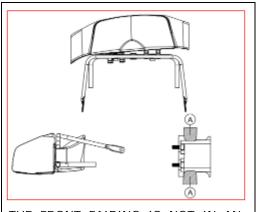
THE FRONT FAIRING IS NOT IN AN ACCEPTABLE POSITION IF ANY PART OF THE TUBES OF THE FRONT BUMPER ARE IN THE AREA 'A'. Where the CIK-homologated detachable front fairing mounting kit is used, it must at all times during live sessions be fitted and maintained in the correct position in accordance with Article 2.3.3 of the FIA Karting General Prescriptions and Technical Drawing 2.2 and 2.2.1.
