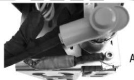
(A) additional ground cable not connected
